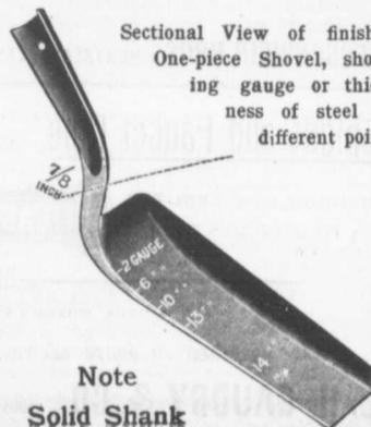
Sectional View of finished One-piece Shovel, showing gauge or thickness of steel at different points
