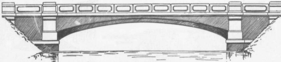
This cut shows ONE of SEVEN arch bridge spans which we are now completing at Ottawa, Ont. All parts including arches and railings are in concrete thoroughly reinforced with steel bars imbedded in same. This construction is very rigid under heaviest loads, and will resist any flood or ice flow. No painting or maintenance; they are there to stay as long as the native rock. Cost about same as for steel bridges, and superior beyond comparison. Plans and tenders promptly submitted.
