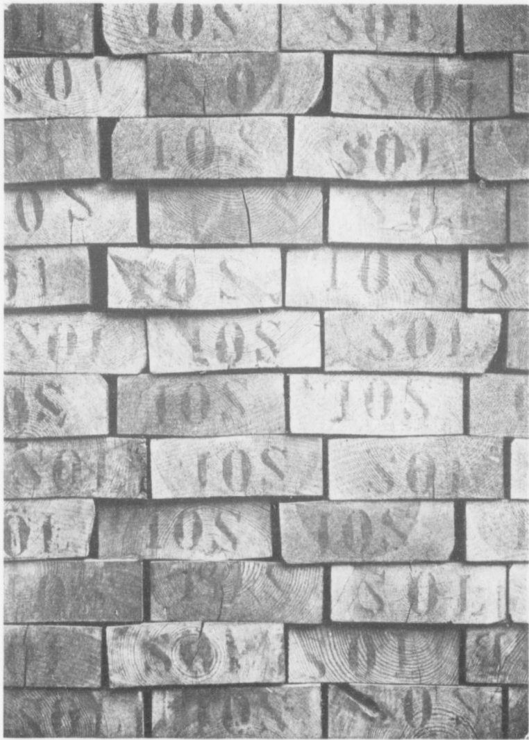
An end view of third grade 3 in. x 9 in. Swedish red deals, used largely in Australia, Africa and the United Kingdom for building and joiner. All Scandinavian and Russian timber is branded in this manner. Many deals are wane covered and nearly all contain heart.
