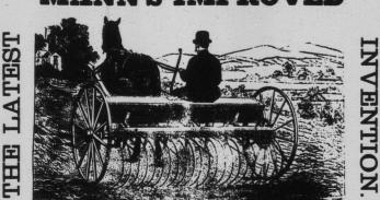
BROAD CAST SOWING ATTACHMENT TO HORSE RAKES, WITH ONE BOX, WITHOUT CHANGE OF GEAR.
