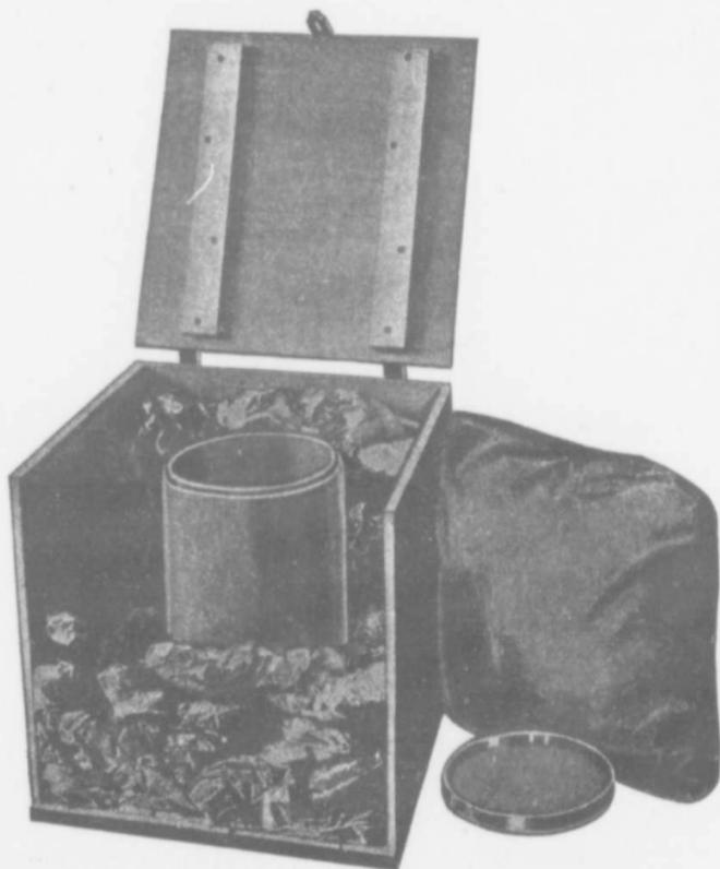
FIG. 40.—Fireless cooker, showing method of packing with paper.
