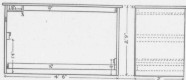
FIG. 29.—Working drawing of cabinet.
