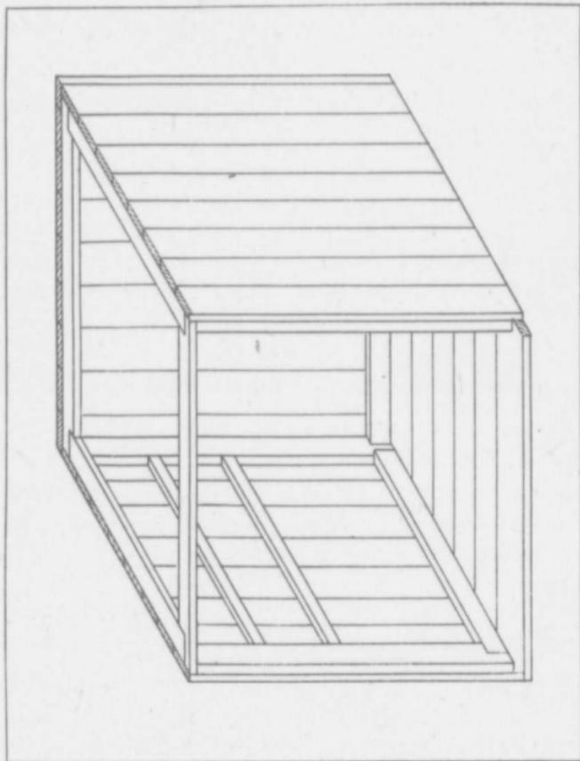
Fig. 35.—Frame of cabinet nailed together
