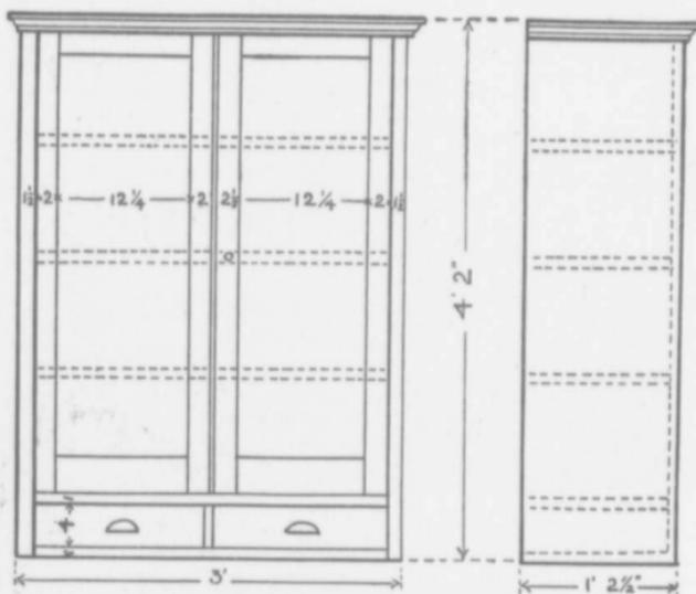
FIG. 28.—Working drawings of cupboard
