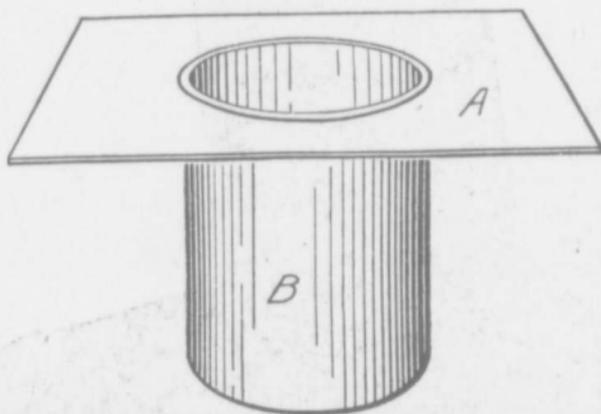
FIG. 41.—Metal lining with rim
