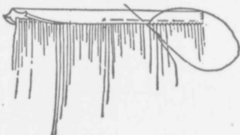
FIG. 16.—Sewing on the belt of the apron
