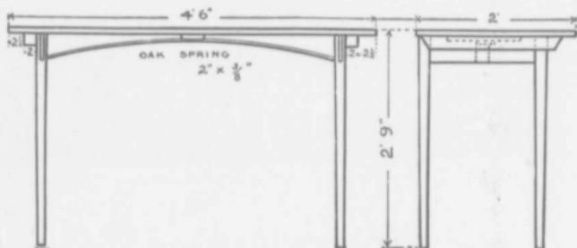
FIG. 22.—Working drawing of folding table
