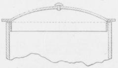
FIG. 42.-Tightly fitting lid
