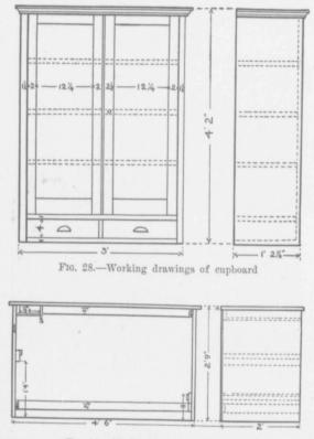
FIG. 29.-Working drawing of cabinet.
