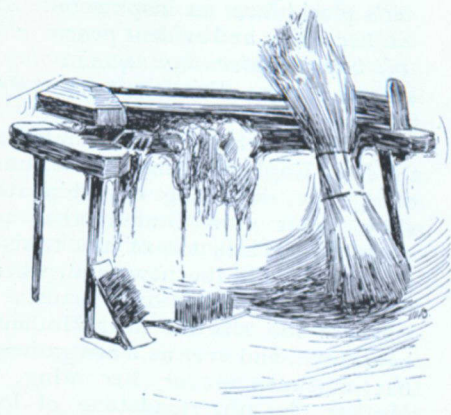
A MACHINE FOR BREAKING THE FLAX— USUALLY KNOWN AS A HACKLE.
