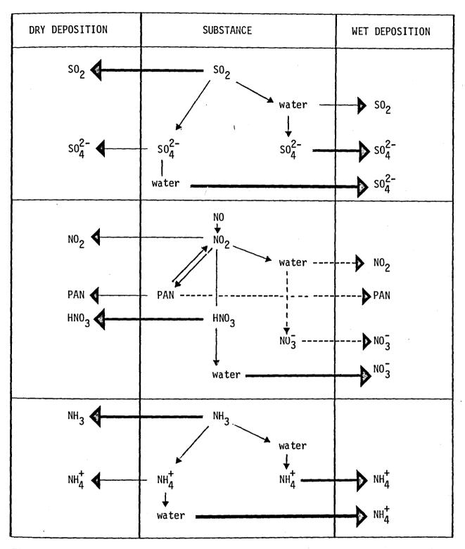
Figure 5.2 Schematic diagram of possible deposition pathways for the major acidic species. The middle column depicts processes or steps along the pathway prior to deposition. The horizontal arrows depict deposition processes for the various species: to the left indicates dry deposition; to the right indicates wet deposition. Heavy lines represent important pathways and broken lines represent uncertain ones.
