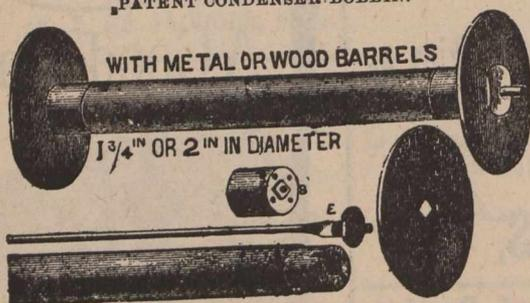
The Heads of these Bobbins contain a Square Hole in the centre, and are fitted on a Square Projection attached to the end of the Barrel, as shown above; thus the heads cannot turn round or get loose. This is the only means of avoiding the frequent and costly repairs, and the abundance of Loose Bobbin Ends so common in Mills. Old Bobbin Ends may be utilized and converted to this principle.
