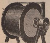
For extracting Iron or Steel from Borings, Ash-Metals, Glass Seeds, Slag Tobacco, &c.
