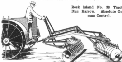
Rock Island Power Disc , in two sizes, 8 and 10 feet. Both Front and Rear Harrow Absolutely Flexible.
