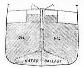
SECTION OF TANK STEAMER, WITH CONICAL EOTTOM.
