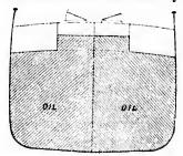
SECTION OF TANK STEAMER WITHOUT WATER-BALLAST BOTTOM. bottom at all. All the same, when bulk transport develops a little more, above all to the East, and vessels on the return voyage are required to bring other cargoes, a reversion to the conical bottom will probably be found necessary, on account of the readiness with which the smooth plating of that form of bottom can be
