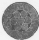
Locked Coil Aerial Cable or Colliery Guide.
