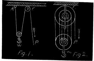
The one end of the rope is made fast at R, then passes over the movable pulley at W and again over the fixed pulley at F. The power is applied at P, to raise the weight suspended from the hook at W which is attached to the movable pulley.
