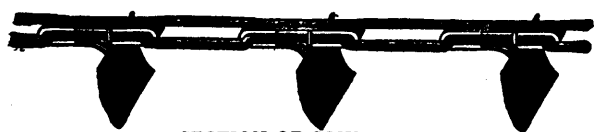
SECTION OF CONVEYOR.
