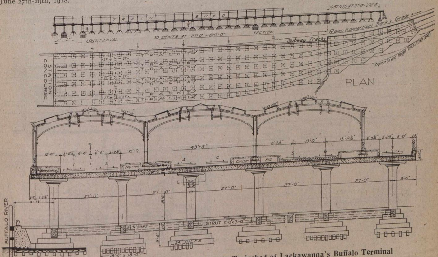
Fig. No. 2—Details of Reinforced-Concrete Flat-Slab Trained of Lackawanna's Buffalo Terminal
