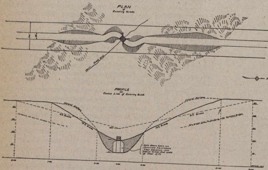
Fig. No. 2—Inadaptable and Unstable Bridge Design
