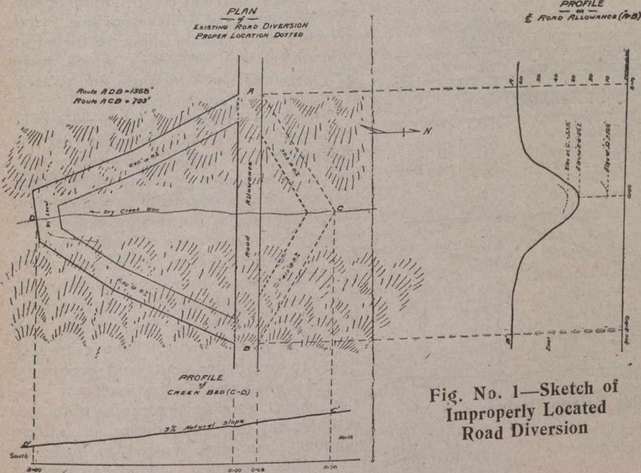
Fig. No. 1—Sketch of Improperly Located Road Diversion
