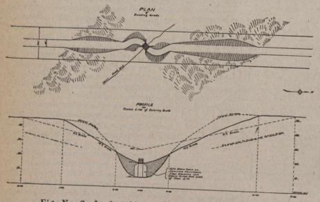
Fig. No. 2-Inadaptable and Unstable Bridge Design
