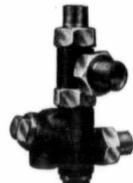
Special high pressure injectors, working up to 235 lbs., can be furnished when desired. The Model "U" lifts water 25 feet; handles water at 130 deg. and delivers to the boiler at almost 212 aeg.
