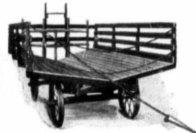
In shock threshing, a big saving can be made by using the racks with the carriers. One Hart Universal and driver will do as much work as two ordinary racks, two drivers and one field pitcher.
