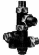
Special high pressure injectors, working up to 235 lbs., can be furnished when desired. The Model "U" lifts water 25 feet; handles water at 130 deg. and delivers to the boiler at almost 212 aeg.
