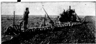
This is the plow double service, as either disc or moldboard bottoms may be used on the same frame.
