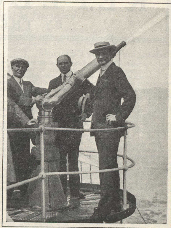
The latest turret nozzle—the most up-to-date feature of the newest fire boats. Mayor Mitchel on right.
