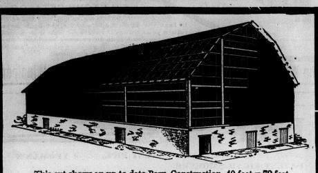
This cut shows an up-to-date Barn Construction, 40 feet x 70 feet, covering with corrugated a The frame work is light, as the corrugated sheets, when nailed in place, make the building very rigid. This drawing is made from actual plans, and the barn has been built many times with splendid results.
