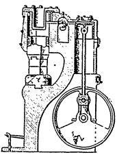
its size. The movement of the treadle which operates the valve is adjustable from one to three inches, responds instantly to touch of treadle, and when the work is not too large the operator can manage both his work and hammer perfectly. A specimen hammer has been creeted and can be seen working at the Dominion Chain Works, 174-176 Front St. E., Toronto,
