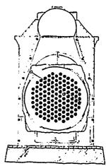
Section at A B showing hand holes and scraper for cleaning tubes.
