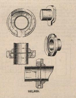
Ing flanged edges tapered from the top to the bottom. The other length of pipe has threaded on the end thereot a flanged member adapted to fit between the projecting lips formed on the other flanged member and is suitably tapered so that when dropped in place the tapered face will wedge against the tapered face of the outer portion of the other flange and consequently draw the two faces of the said flanges tightly together, pressing against the gasket and making the joint secure.
