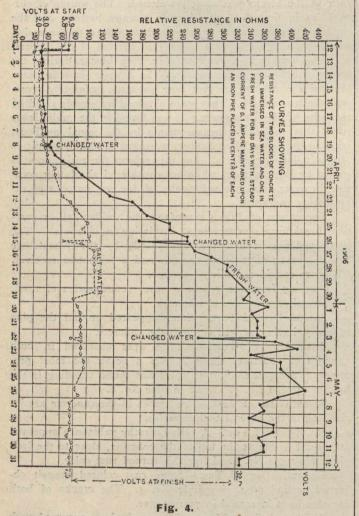
the actual total amount of electrolysis which had occurred. However, all scale that could be readily removed was removed before the final weights were taken.
