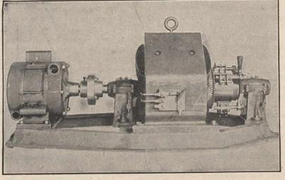
Twenty-five Horse-power Directly Connected to Electric **Generator.**
