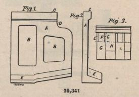
are arranged in pairs, with their angle-irons E facing each other. The distance between each block forming a pair, and between each pair of blocks, may be varied. Between each block A forming a pair there is inserted a stone or other paving sett F which is the same length as the exposed surface of the blocks, but the next abutting sett G is approximately twice the length of the first sett F or of the ordinary size, so as to break joint with the row of setts H on either side.
