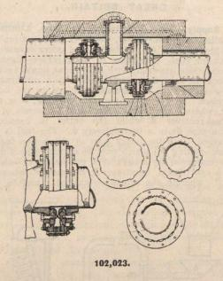
of to limit the outward movement of the expansion flange and extension pipe and sustain a continuous spring pressure on said flanges to make a water-tight joint.
