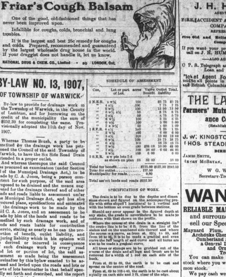
From st 103+40 to 111½, the earth is all to be cas to the south side of the drain, 3 it. clear of the edge From st. 111½ to 112, the earth is to be cast about equally on each side and 3 f. clear of the edge.
