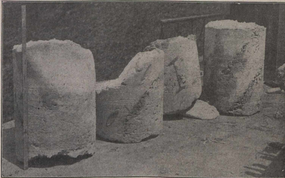
Cores from a 29 inch bore hole. Note water-pipe and eye beam cut clean through.
