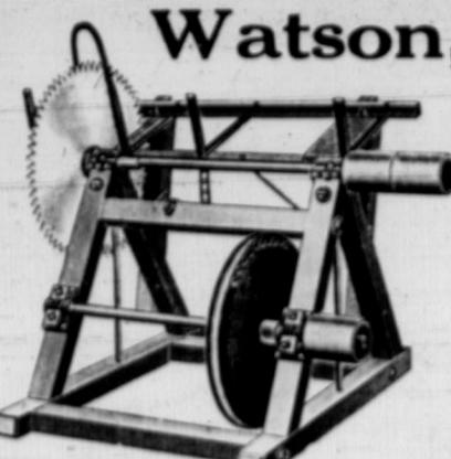
Watson's Pole Saw is of the same high quality of workmanship and material as all other Watson goods. Strongly built, rigid frame which stands firmly and evenly on the ground; equipped with heavy steel shafts and boxes, solid fly wheel and three pulleys. Blade is of finely tempered steel which will "just slip through the wood."
