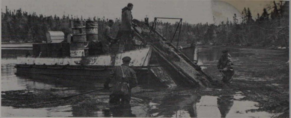
Innovation: A terry cloth conveyor belt developed to pick up Bunker "C" oil spills is one of several new Canadian techniques used in disasters. A conventional snow-blower blasts peat moss over polluted areas to absorb the oil.
