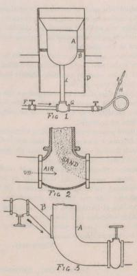
of how to build and use a sand-blast, together with a description of sand sifting apparatus, may be useful to architects and builders. If the sand-blast apparatus is properly built, the force which may be obtained from the stream of fine, hard and sharp grains of sand from the machine is remarkable. The discharge of sand is capable of cutting the hardest of substances.
