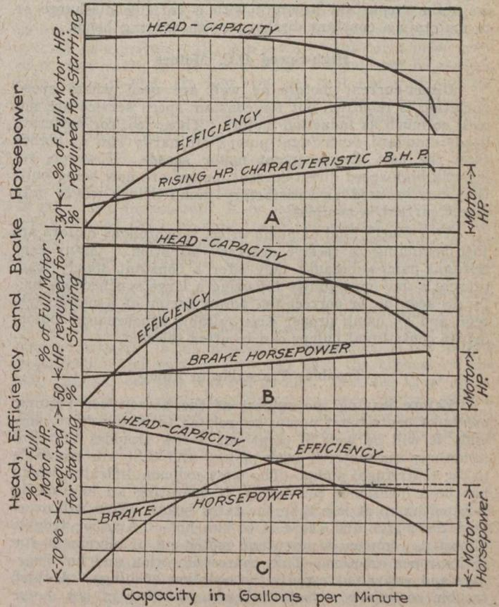
FIG. 1—PUMP CHARACTERISTIC CURVES
