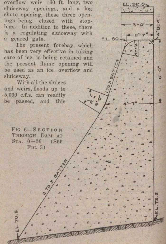
FIG. 6—SECTION THROUGH DAM AT STA. 0+20 (SEE FIG. 3)
