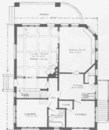
FIRST FLOOR PLAN— CONCRETE BUNGALOW—#3025
