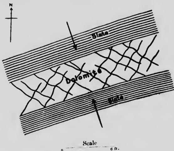
FIG. 3. Relation of fractures in dolomite to direction of stress.
