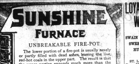
the upper portion expands much more than the This uneven expansion causes a strain too great for a one-piece fire-pot to stand.
