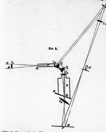
color to be matched. The other half, as a prismatic spectrum, illuminates a piece of standard white paper placed beside the colored surface. By an ingenious shutter arrangement the spectral colors are used for matching and then determining the color composition of the beam.
