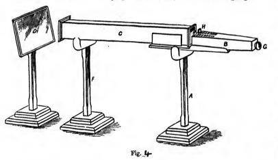
cells at H on either side. Light is taken from the standard white reflector, D, on stand D B C, for transmission through the tubes to the eye-piece.
