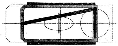
Ovals and Ellipses.—Fig. 6.—Suggestion of an Instrument, Working on the Principle of a Connecting Rod, which may be made to Produce Perfect Ellipses.
