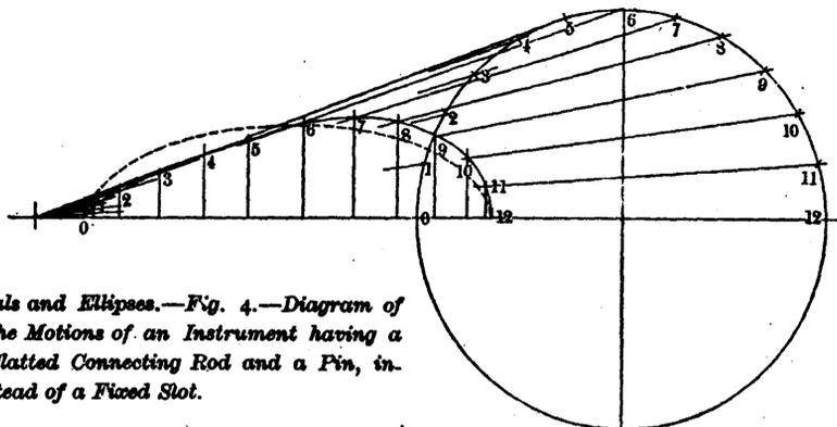
Ovals and Ellipses.—Fig. 4.—Diagram of the Motions of an Instrument having a Slatted Connecting Rod and a Pin, instead of a Fixed Slot.
