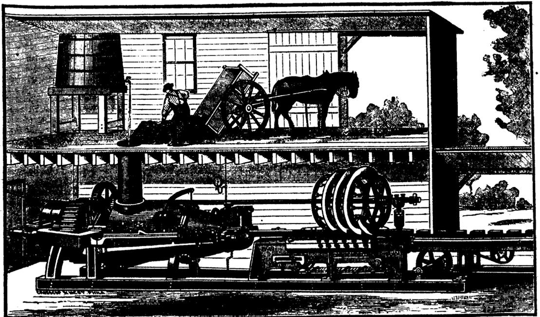
Fig. 1.—PERSPECTIVE VIEW OF THE CHAMBERS "B" BRICK MACHINE.—(SEE NEXT PAGE.)
