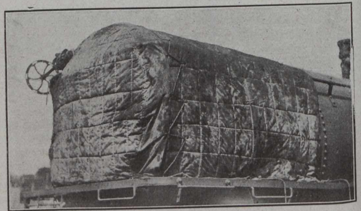
Insulating Cover Partly in Place on Asphalt Tank Car. This New Cover Reduces Time of Unloading the Car.
