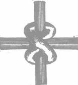
The Anthony is made from all No. 9 spring steel wire, which is thoroughly galvanized.
