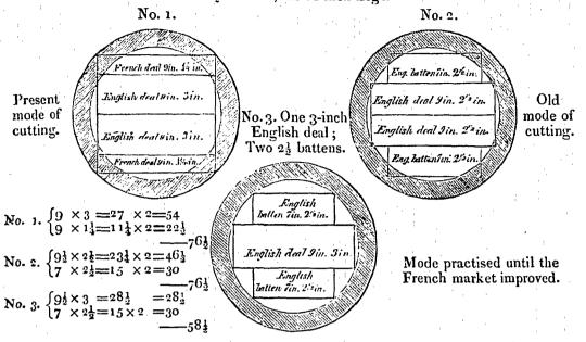
Proportions of Timber, supposing the Logs to be measured with a Calliper.
