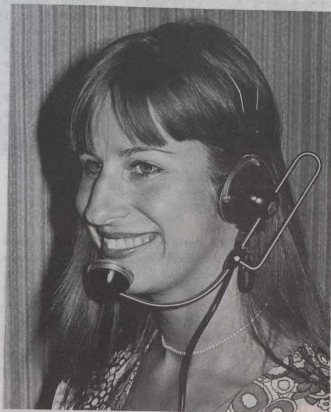
Old headset weighs about half a pound and requires a headband. Background noise can create problems.
