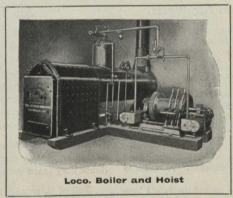
When boiler and engine are connected in the manner here shown, little steam is lost by condensation, even in winter
