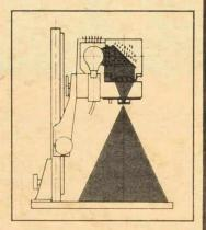
does not go straight from lamp to negative, but is deflected downwards by a mirror. Heat escapes not only through lamphouse vents but also from back of mirror. Lamp may be raised and lowered, as well as rotated to ensure precise centering with mirror. Illumination is totally even, yet retains the crispness of a condensor enlarger
