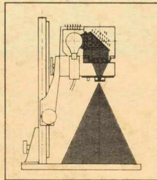
does not go straight from lamp to negative, but is deflected downwards by a mirror. Heat escapes not only through lamphouse vents but also from back of mirror. Lamp may be raised and lowered, as well as rotated to ensure precise centering with mirror. Illumination is totally even, yet retains the crispness of a condenser enlarger.
