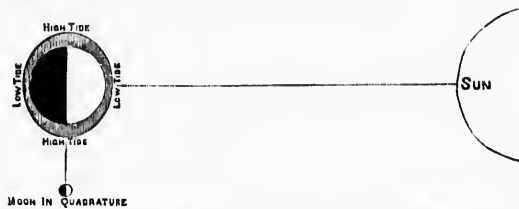
FIG. 22.—NEAP TIDES; attraction of moon and sun at right angles; the moon tide being higher than the sun tide.
