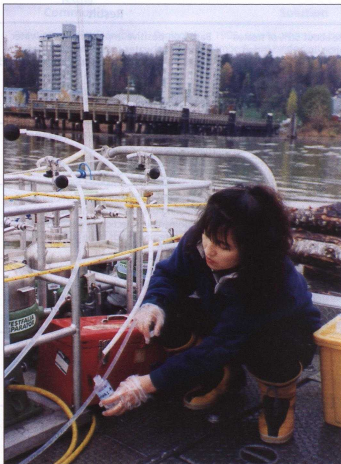
Sampling water and suspended sediment from the Fraser River in British Columbia for the Fraser River Action Plan sediment quality study. Photo credit: Aquatics Section, Pacific and Yukon Region, Environment Canada.
