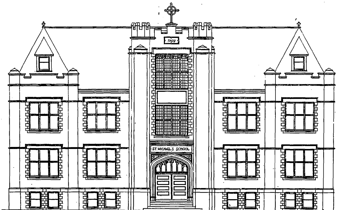
FRONT ELEVATION, ST. MICHAEL'S PARISH SCHOOL, BELLEVILLE, ONT., SHOWING DETAIL OF CENTRAL TOWER, MAIN ENTRANCE AND WINDOWS. MR. C. P. MEREDITH, ARCHITECT.
