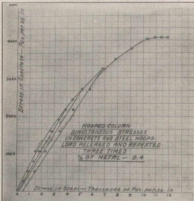
Fig. 7.—Curve showing the behaviour of a 1:1 hooped concrete under repeated compressive stresses.
