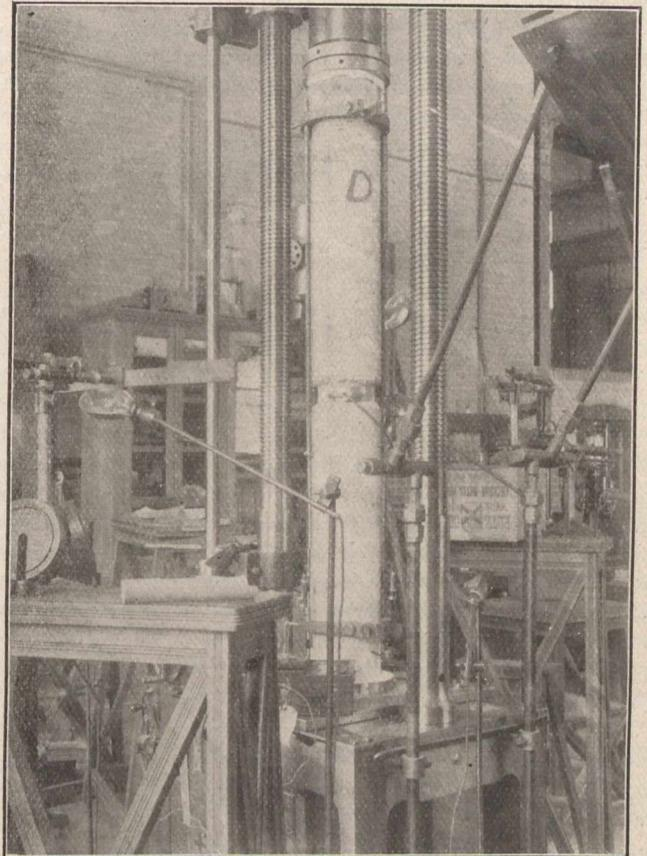
Fig. 10.—Hooped column under test.
