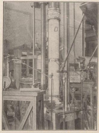
Fig. 10.-Hooped column under test.
