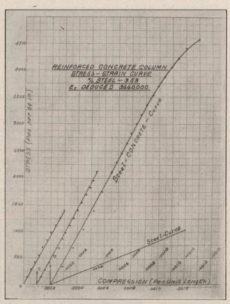
Fig. 3.—Curve showing the behaviour of a 1:1 concrete column with longitudinal reinforcement, under compressive stress.
