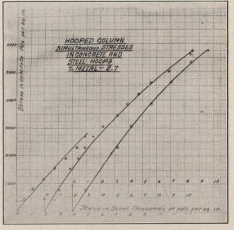
Fig. 8.—Gurve showing the ratio of steel stress to axial compressive stress in hooped concrete mixture 1:1.
