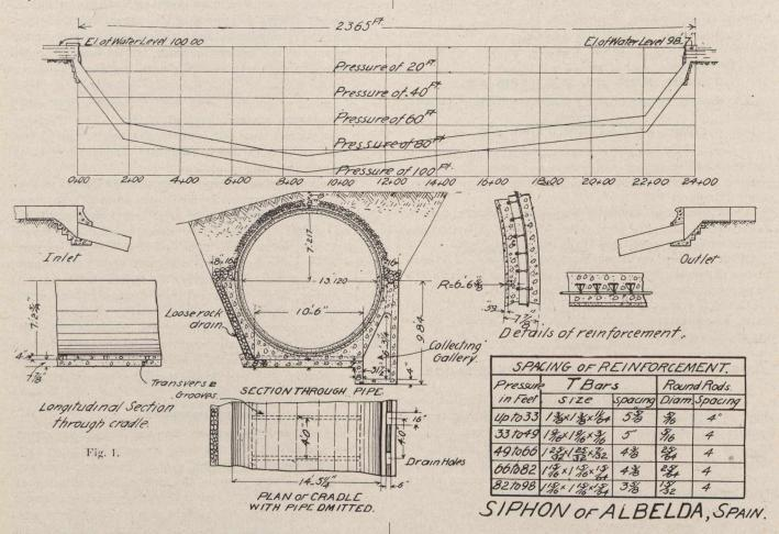
conduit would find an easy passage into the drains. The concrete used consisted of about 1 part of cement to 41/4 of sand and 8½ parts of gravel passed through a 2¾-inch screen.
