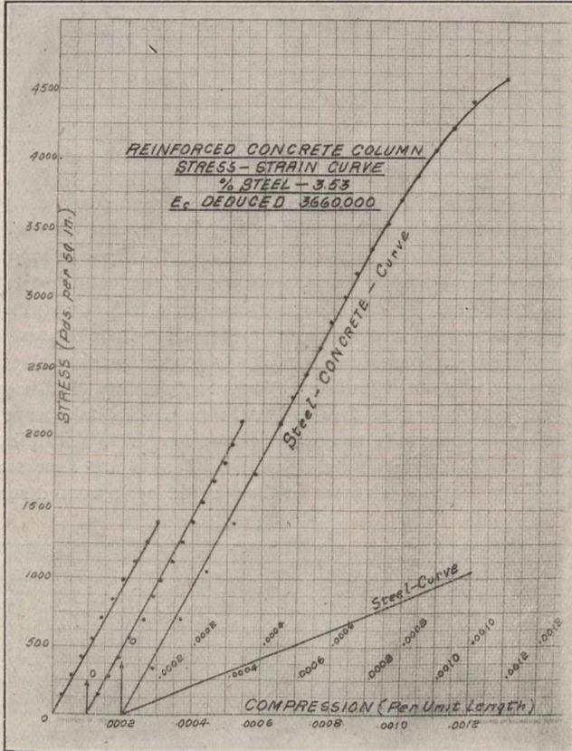
Fig. 3.—Curve showing the behaviour of a 1:1 concrete column with longitudinal reinforcement, under compressive stress.
