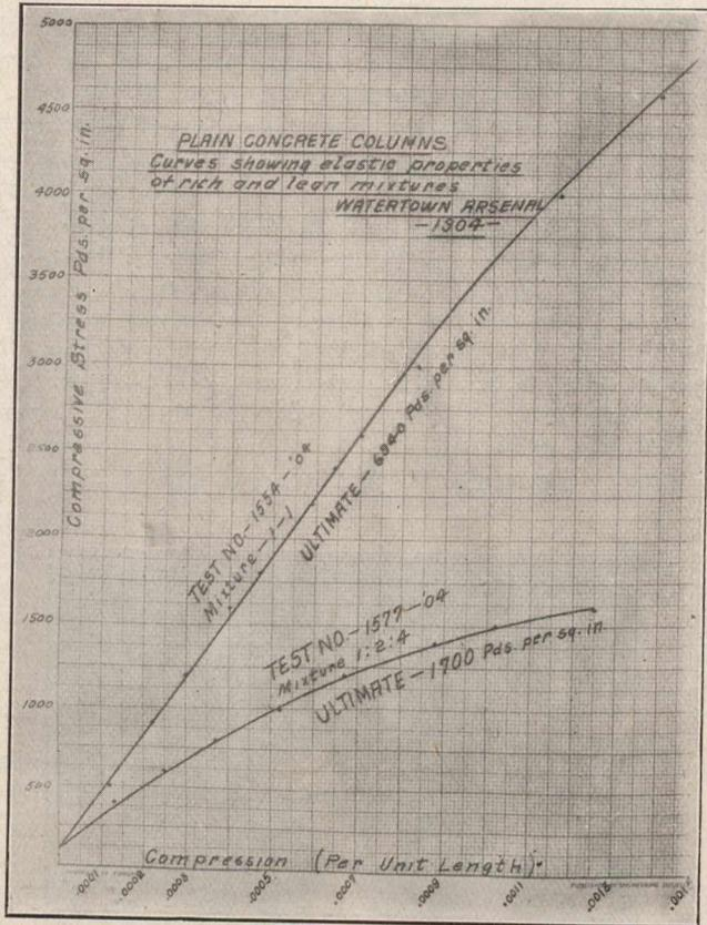
Fig. 1.—Curve showing the behaviour of typical rich and lean mixtures under compressive stress.
