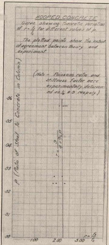
Fig. 9.—Curve showing the theoretic variation of the ratio  $f_s/f_c$  with change in the percentage of metal in hooped concrete of mixture 1:1.
