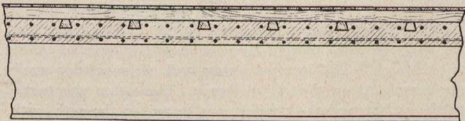
*Wood Top Reinforced Concrete Floor Designed by
