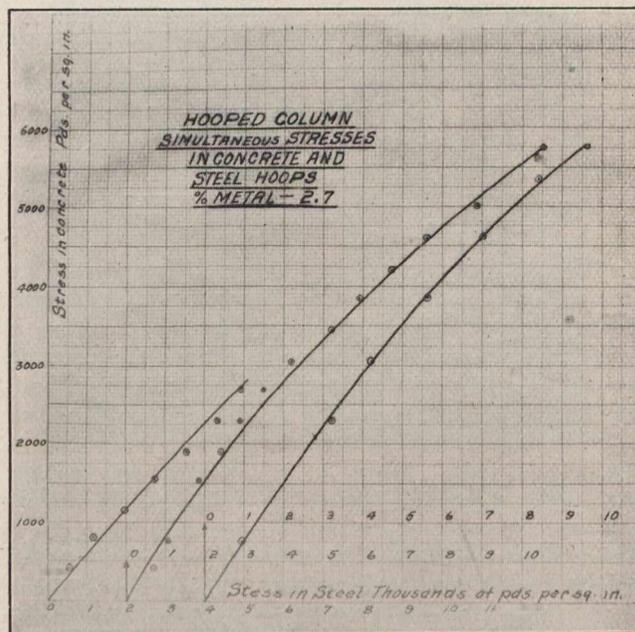
Fig. 8.—Curve showing the ratio of steel stress to axial compressive stress in hooped concrete mixture 1:1.
