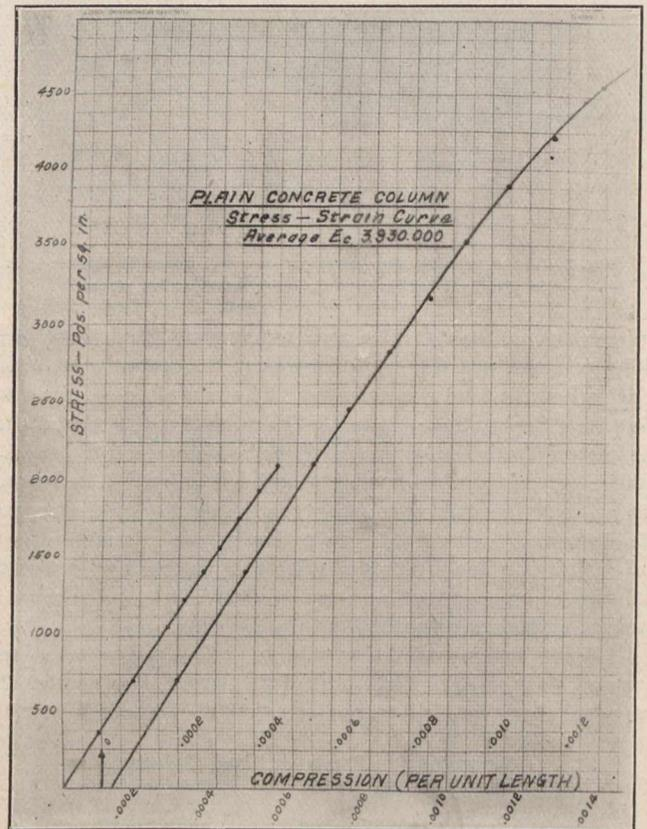
Fig. 2.—Curve showing the behaviour of a 1:1 plain concrete under compressive stress.
