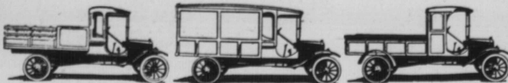
Three of the many body styles that may be mounted on the Ford truck chassis
