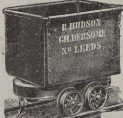
76—R. H.'s Patent Steel Mining Wagon
